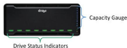
**Figure 2.** Drive status indicators exist for each drive and a capacity gauge shows what percentage of overall capacity is currently being used.
