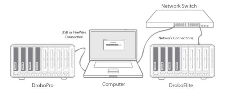
In general, you **cannot** migrate data by moving hard drives from the DroboPro to the DroboElite. You will need to **copy the data from the DroboPro to the DroboElite**.
