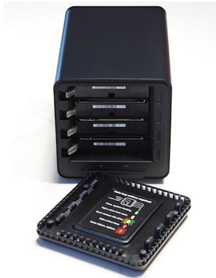
There are blue LEDs along the bottom of the drive that indicate percentage capacity during startup, as well as a status LED for each drive. Power is supplied by a "brick" with a six-foot cable.
